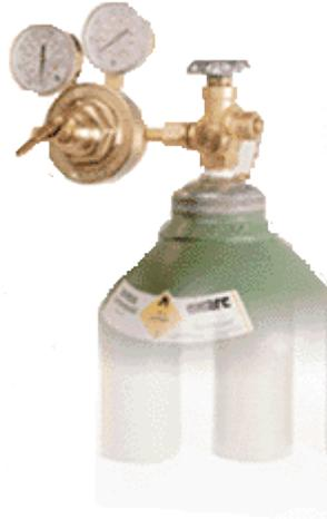
If there is any question as to the suitability of a regulator for a particular gas, check with your vendor for advice. After the regulator is attached, the cylinder valve should be opened just enough to indicate pressure on the regulator gauge (no more than one full turn) and all the connections checked with a soap solution for leaks. **Never use oil or grease on the regulator of a cylinder valve.**
