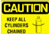
**Gas cylinders must be secured at all times to prevent tipping.**
